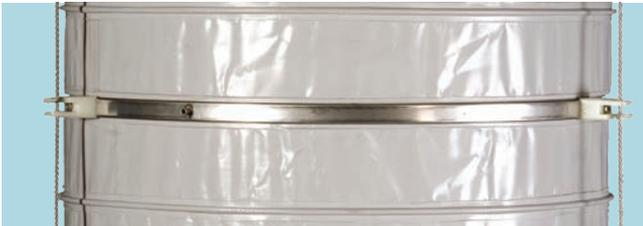
For food products a PVC-clad polyester module in a light grey colour can be used. The material is approved for drinking water, and can thus be used with all kinds of foodstuffs, provided that the product temperature does not exceed 70°C. The module is also resistant to UV light, rot and fungus.
