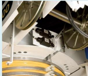
The motor winch is equipped with three sturdy winch drums as standard, supported by a high-quality ball bearing. The three corresponding hoisting wires give extremely even and balanced hoisting and lowering. A tight/slack wire function is provided as standard on all loading chutes.
