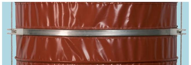
The red module material is Valmex Corotex P250, a rusty-red polyester and fibre glass fabrics coated with silicone rubber on both sides. The type R module has a continuous working temperature area ranging from -40°C and 150°C with short term working temperature on 220°C.
