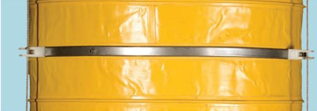
The standard module for Moduflex loading chute is in PVC-clad polyamide with the designation PA700, in a yellow colour code. This module may be utilised with many different products, provided that the product temperature does not exceed 70°C.
