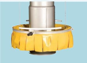
For tanker truck loading, the dust skirt is raised and fastened using the fittings on the two handles. The outlet cone has a similar design to that of the tank outlet.
