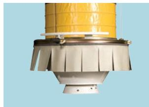
For tanker loading, the dust skirt is raised and fastened using the fittings on the two handles. The outlet cone has a similar design to that of the tank outlet. An electrical raising/lowering function of the skirt is available as an option.
