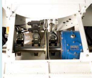
The motor winch is supplied with a gear motor. It can be supplied with a control panel in which all functions are integrated, or with a junction box. The control cabinet or junction box is mounted on sliding brackets which enable the control gear to be lowered for easy access.
