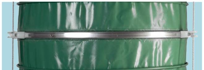
In conditions, where there is a possibility for very low air temperatures, a special material has been developed, from which these green modules are manufactured. The module material is Vinyplan Artic with a base material of polyester and a PVC/PU coating. The type Z module has a temperature working range from -60 °C - +70 °C. At the same time, this material is anti-static as standard.
