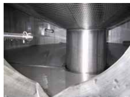
Fluid bottom with integrated spray ball for cleaning of the clean-air section
