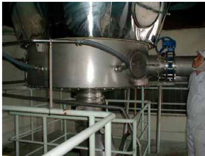
The Simatek fluid bottom ensures an easy discharge, even in case of a bridging powder type
