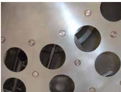
SimPulse 3C tube sheet with integrated CIP nozzles for cleaning of the bag outside and the product-side of the filter chamber
