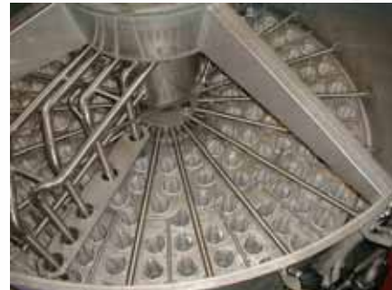
SimPulse 3C indexing nozzle system for wet cleaning of the bag inside as well as the clean-air chamber
